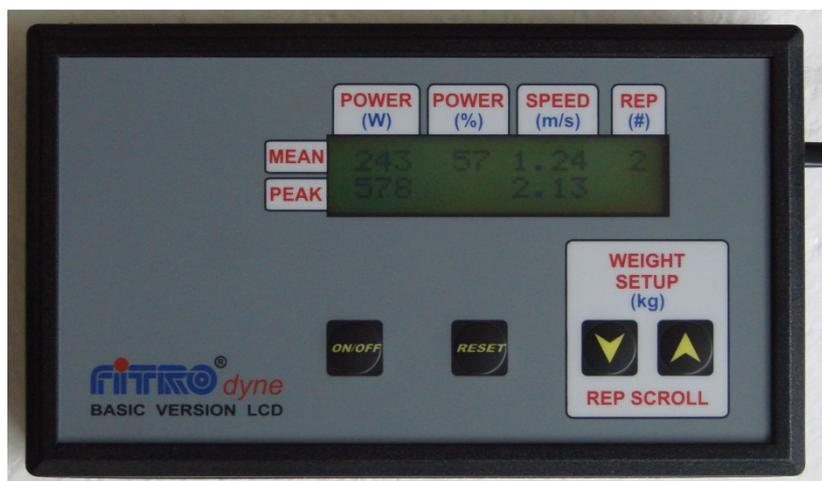
The data (mean and peak values of power and speed from concentric phase of corresponding repetition) are displayed automatically after finishing concentric (upward) phase of single repetition. Also % values (mean power from concentric phase) of the best repetition in particular set (since pressing reset) is updated in the second column from the left.
