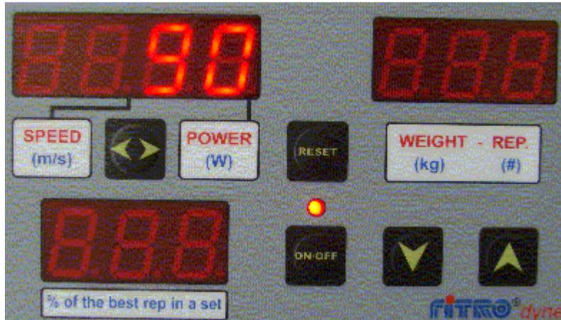
Further pressing of RESET opens the routine in which one can the limit for the sound signal (a double beep) that will occur after each repetition in which the power exceeds the limit. Power above this limit will be indicated by double beep. Setting 99% limit, the double beep will indicate the best value in current set. Setting 100 % limit disables this feature..
