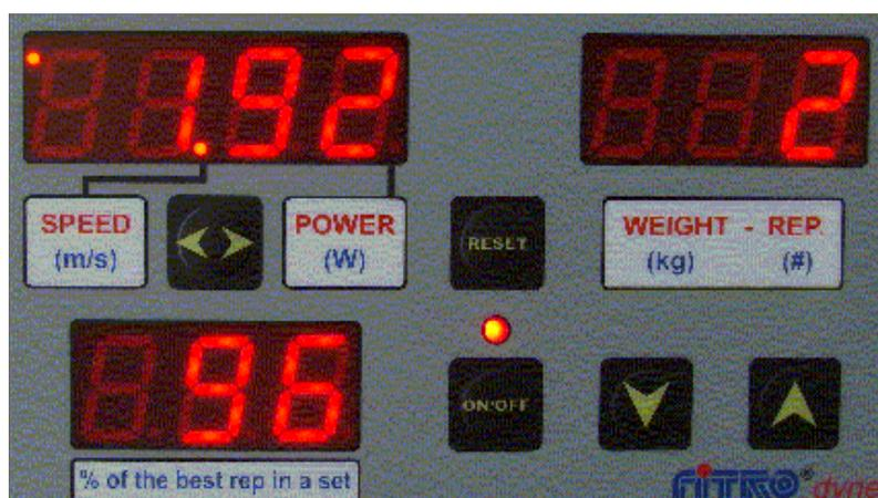
Use **▼** **▲** buttons to go through reps from the current series. RESET button will end up a series and the device will be set to the starting mode expecting new weight to be set. Data from previous set remains stored in the internal memory of display unit, however cannot be displayed. However, they can be transferred to the PC by using the interface.
