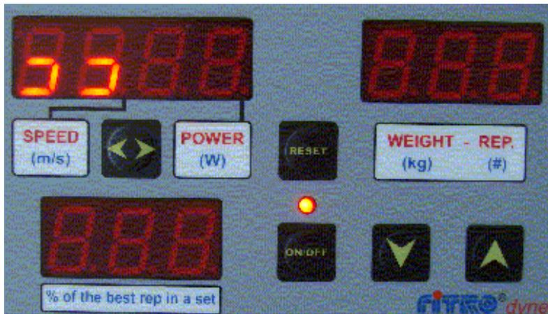
After transferring data from memory to the PC, CC (**clear data**) will show up on the display. For erasing memory you need to press ▼ ▲ buttons at the same time. If you return to the weight setting mode by pressing RESET data from previous set (sets) will remain the internal memory.
