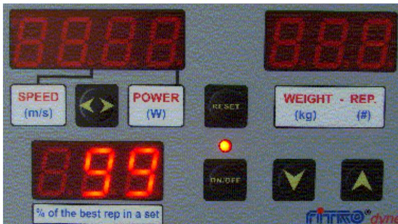
Further pressing of RESET opens the **SEND DATA** routine. To send data from the device's internal memory to your PC through interface one has to press ▲, or enter the weight setting mode by pressing RESET button.
